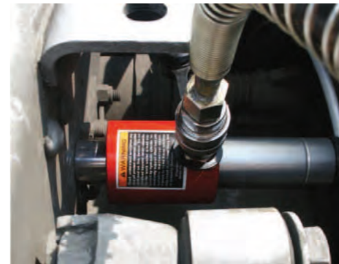
▲ Press truck wheel from nave with the mini-press. Fits between the chassis and wheel.
