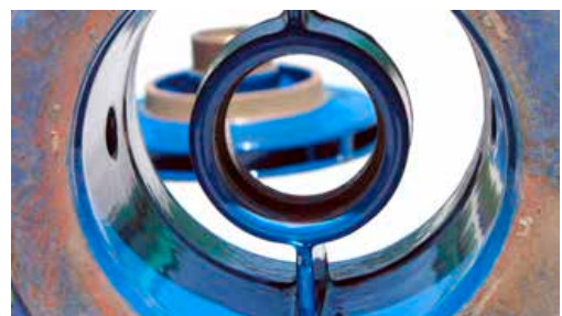
... and that's how it should be! The MetaLine® surface regeneration is significantly smoother than casted steel and up to 500 % more wear-resistant. Repairs at least as durable as an original spare part – but lower in costs ...
